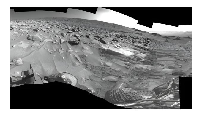
NASA's Curiosity left several sets of tracks where the rover experienced a fault, or unexpected stoppage mid-drive, while attempting the most difficult climb the mission has faced: a slope with a sharp 23-degree incline, slippery sand, and wheel-size rocks. Credit: NASA/JPL-Caltech
