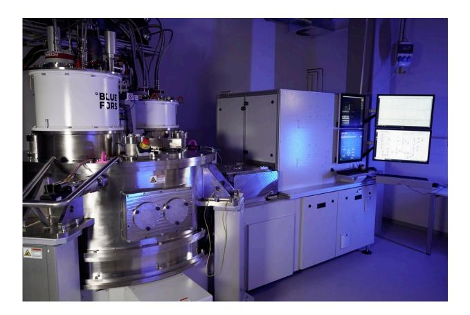
The cryogenic on-wafer prober at Fraunhofer IAF enables fully automatic characterizations of up to 25 whole 200-mm or 300-mm wafers with devices for quantum computing and sensing. Credit: Fraunhofer IAF
