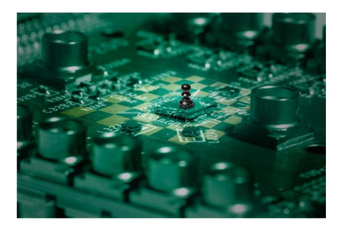
Photograph of the quantum chip hosting the 16 quantum dot crossbar array, seamlessly integrated to a chessboard motif. Every quantum dot, like a pawn on a chessboard, is uniquely identifiable and controllable using a coordinate system of letters and numbers. Photo credit: Marieke de Lorijn for QuTech. Credit: Marieke de Lorijn for QuTech
