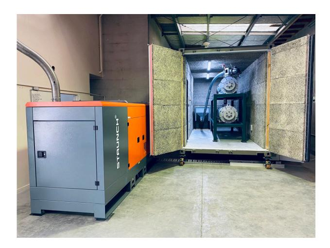
Heavily modified shipping containers at EDL's research and development facility in Henderson, Auckland, house the company's patented Mechanochemical Destruction (MCD) reactors. Credit: EDL Ltd
