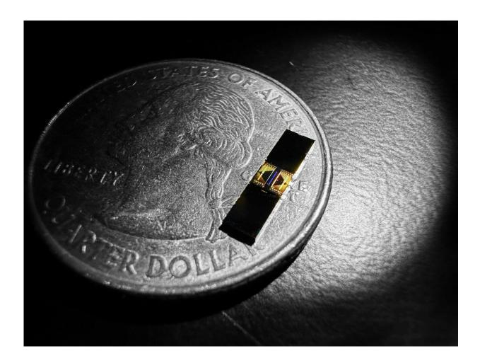
Researchers have shown that dissipative Kerr solitons (DKSs) can be used to create chip-based optical frequency combs with enough output power for use in optical atomic clocks and other practical applications. The advance could lead to chip-based instruments that can make precision measurements that were previously possible only in a few specialized laboratories. Credit: Grégory Moille, Joint Quantum Institute, NIST/University of Maryland
