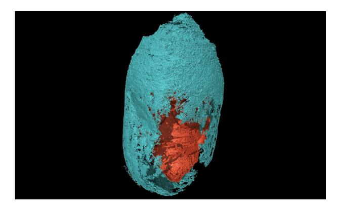
X-ray micro-computed tomography views of a male Eucera bee (ventral) inside a sealed cocoon. View obtained in the ICTP ElettramicroCT, Trieste's Elettra synchrotron radiation facility in Italy. The image shows the architecture of the excavated brood chamber closed by the spiral cap, containing an adult bee close to abandoning the cell. Credit: Federico Bernardini/ICTP.
