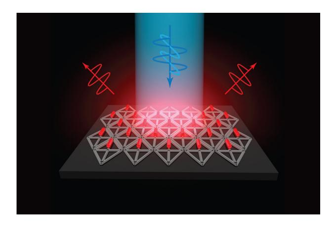
MIT engineers have used DNA origami scaffolds to create precisely structured arrays of quantum rods, which could be incorporated into LEDs for televisions or virtual reality devices. Credit: Dr. Xin Luo, BatheBioNanoLab
