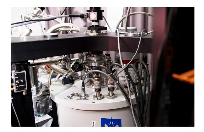
The cryogenic superconducting magnet where electrical measurements were taken in the experiments at Nanyang Technological University, Singapore. Credit: NTU Singapore
