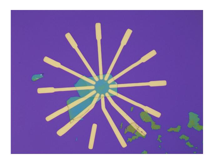
A microscopic image of the tiny device containing antiferromagnetic manganese bismuth telluride (green) that the Nanyang Technological University, Singapore researchers did their experiments on. The lines (light yellow) radiating from the center are electrodes from which current was passed through the manganese bismuth telluride. Credit: NTU Singapore
