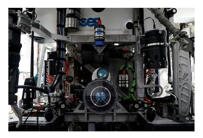
The main camera of the remote operated dive vehicle Deep Discoverer is visible aboard the NOAA Okeanos Explorer, Friday, June 23, 2023, in Kodiak, Alaska. The vehicle, which is designed to explore the deep sea and sea floor, can reach depths of up to 6,000 meters (19,685 feet). Credit: AP Photo/Joshua A. Bickel
