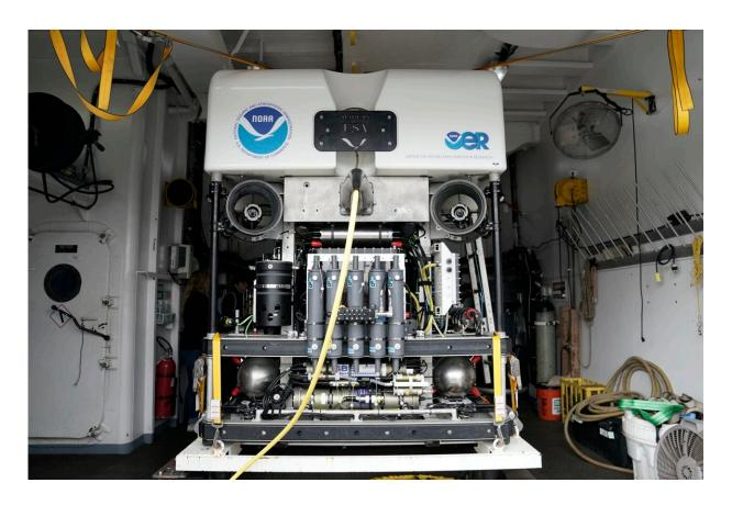
The remotely operated dive vehicle Deep Discoverer is visible aboard the NOAA Okeanos Explorer, Friday, June 23, 2023, in Kodiak, Alaska. The vehicle, which is designed to explore the deep sea and sea floor, can reach depths depths of up to 6,000 meters (19,685 feet). Credit: AP Photo/Joshua A. Bickel
