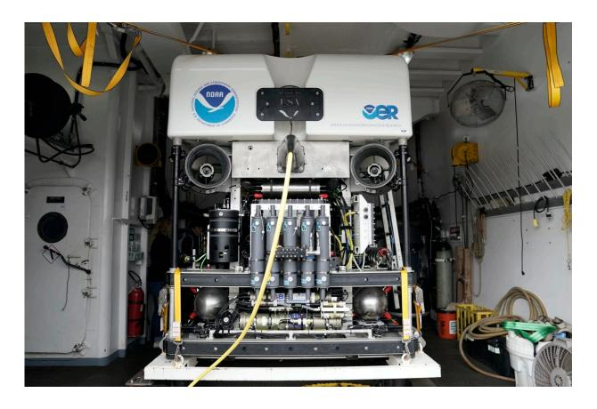
The remotely operated dive vehicle Deep Discoverer is visible aboard the NOAA Okeanos Explorer, Friday, June 23, 2023, in Kodiak, Alaska. The vehicle, which is designed to explore the deep sea and sea floor, can reach depths depths of up to 6,000 meters (19,685 feet). Credit: AP Photo/Joshua A. Bickel
