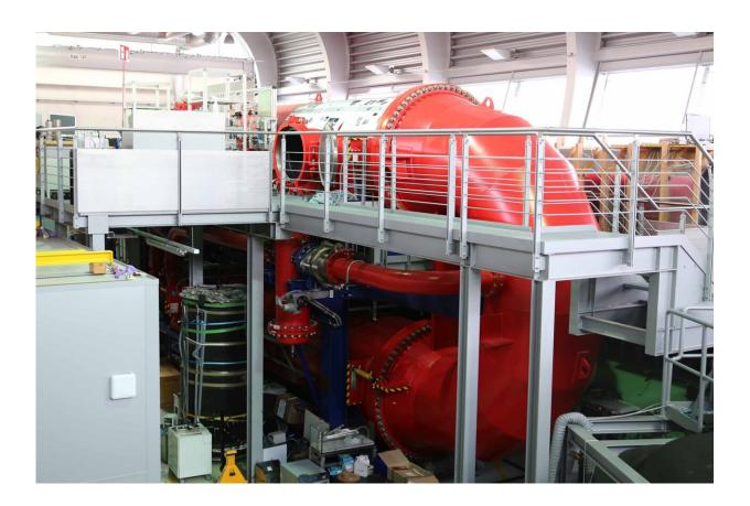
The wind tunnel at MPI-DS allows to generate very high degrees of turbulence at high pressure to measure different flows. Credit: Max-Planck-Institut für Dynamik und Selbstorganisation
