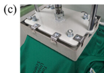
(c) Apply heat and pressure
