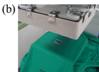
(b) Set the sensor on textile
