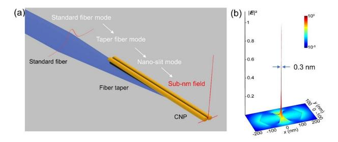
Waveguiding scheme to generate a sub-nm-confined optical field in a nano-slit mode. (a) Schematic illustration of the CNP waveguiding scheme. (b) 3-D plot of the cross-sectional field intensity distribution of the nano-slit mode. Credit: *Advanced Photonics* (2023). DOI: 10.1117/1.AP.5.4.046003
