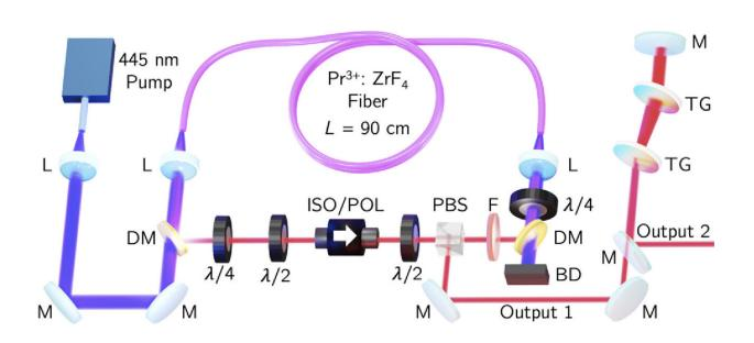
Experimental setup of the fiber laser. BD, beam dump; DM, dichroic mirror; ISO/POL, polarizing optical isolator; L, lens; M, mirror; PBS, polarizing beam splitter; TG, transmission grating; ?/2, half-wave plate; ?/4, quarter-wave plate. Credit: *Optics Letters* (2023). DOI: 10.1364/OL.492671
