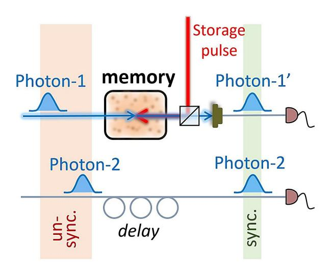
Photon-1 and photon-2 are generated at random times from the photon source. Photon-1 is stored in the quantum memory with a storage pulse, while photon-2 enters into an optical fiber delay-line. Subsequently, photon-1 is retrieved from the memory synchronously with photon-2 by application of the second, retrieval,
