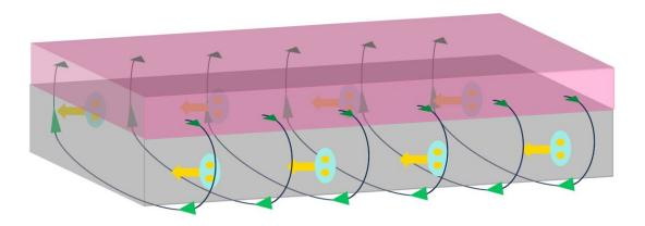
MIT scientists and colleagues have created a superconducting device that could dramatically cut energy use in computing, among other important applications. In one design the diode consists of a ferromagnetic strip (pink) atop a superconducting thin film (grey). The team also identified the key factors behind the resulting current that travels in only one direction with no resistance. Credit: A. Varambally, Y-S. Hou and H. Chi
