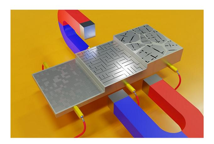
3D model: A single-crystalline sample of the Heusler compound, tailored by means of ion beams with graded thickness, is shown. Magnetic domain structures (black lines) form under the influence of the magnetic field. Credit: B. Schröder/HZDR
