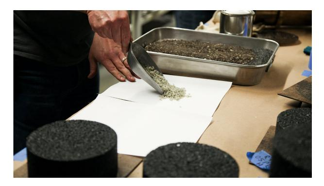
Lab staff in the Mizzou Asphalt Pavement and Innovation Lab show the plastic waste particles that are being added to the pavement mixture. The lab is located inside the University of Missouri College of Engineering. Credit: University of Missouri
