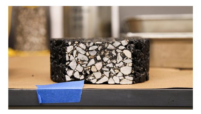
An asphalt pavement test mixture sample designed by the Mizzou Asphalt Pavement and Innovation Lab is ready for further lab testing to determine its strength and durability. Credit: University of Missouri
