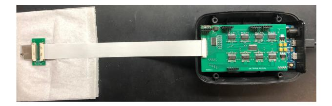
This photo shows a test setup. The sensor is on left, and it is connected to a small circuit board. A long strip connects that to a larger cellphone-sized circuit board incased in plastic. Credit: MIT researchers
