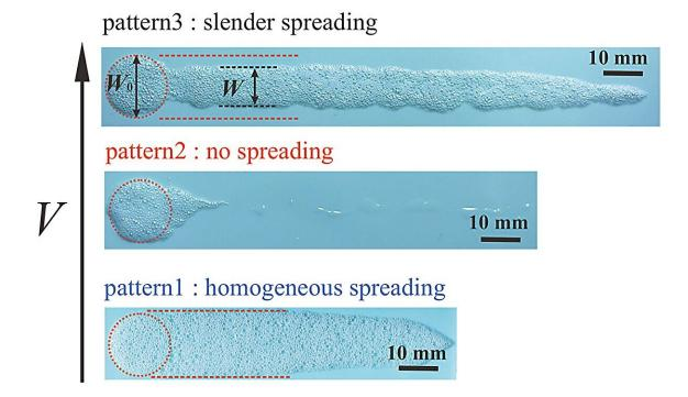
As the plate speed is increased, the foam is no longer spread evenly, but drifts along on a sheet of liquid. At even faster speeds, a thin trail of foam is left behind. Credit: Tokyo Metropolitan University
