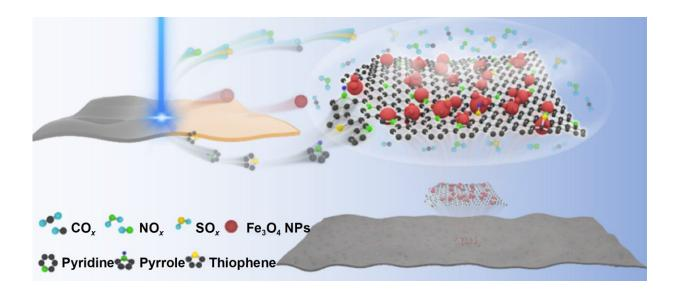
When a short-wavelength laser interacts with a coated material, both photochemical and photothermal reactions takes place resulting in material chemical and physical changes leading to new functional surfaces. Credit: *International Journal of Extreme Manufacturing* (2023). DOI: 10.1088/2631-7990/acdb0c
