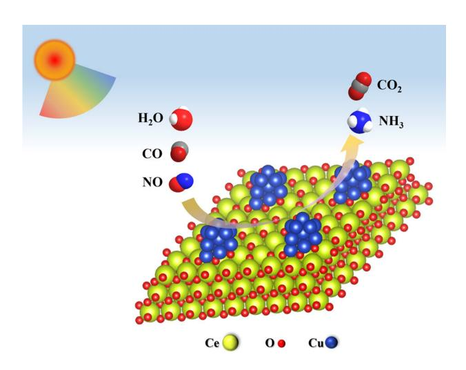
$NH_3$  is not only the key chemical raw material for the industry but also a carbonfree fuel and mobile carrier of renewable energy. In the NO-CO-H2O reaction, NO is reduced to  $NH_3$  by CO and  $H_2O$  over  $Cu/CeO_2$  under mild conditions. The visible-light-induced local surface plasmon resonance (LSPR) effect of Cu promotes the reactivity and selectivity of  $NH_3$ . Credit: Chinese Journal of
