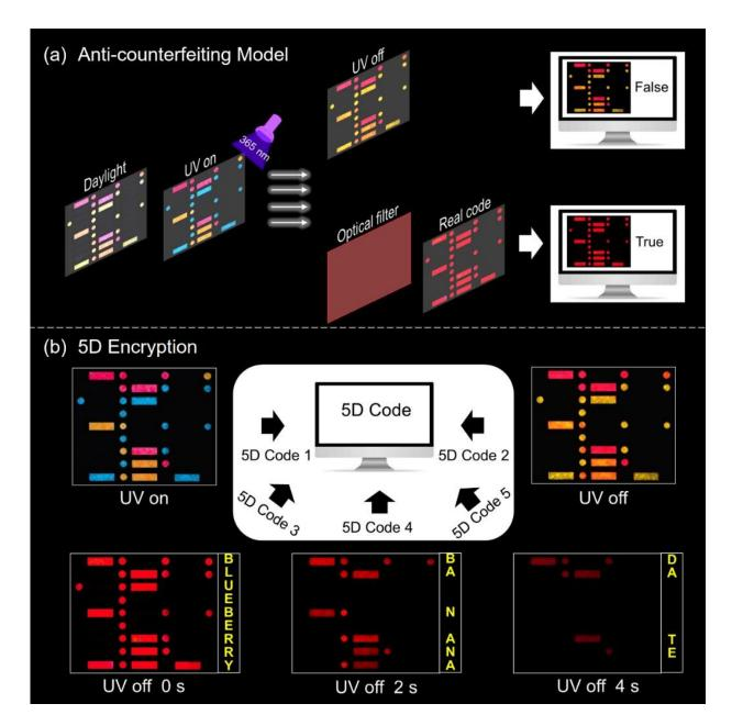
(a). Schematic diagram of the structure of the anti-counterfeiting model; (b). Initial code information composed of three materials under 365 nm UV light (5D Code 1) and after removal of the UV light (5D Code 2), and the 5D Code 3, 4, 5 information that changed with time was observed after using with the optical filter ( $\lambda_{cut-off} = 600$  nm). Credit: SIBET
