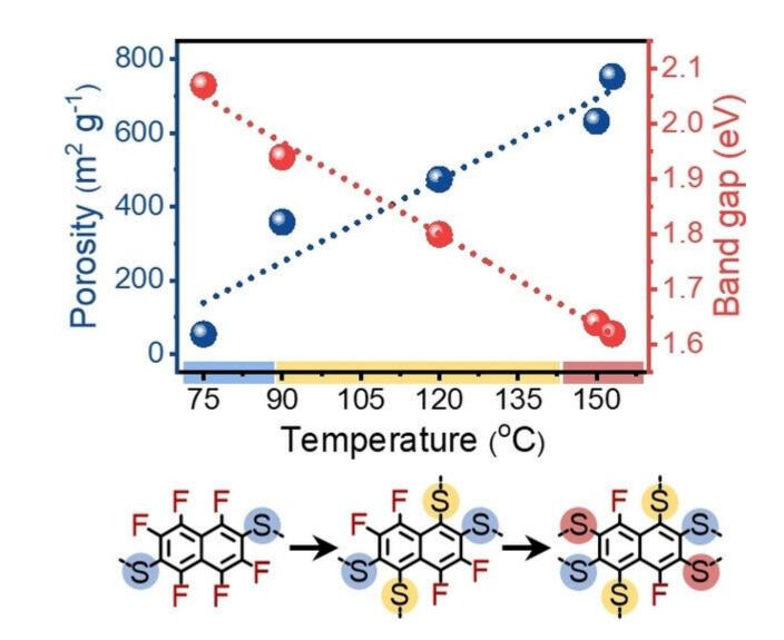
A conventional polycondensation reaction can provide the simplest route to generating porous poly(aryl thioether)s. Controlling the temperature orients the reaction toward the regioselective multi-substitution of aryl fluorides,
