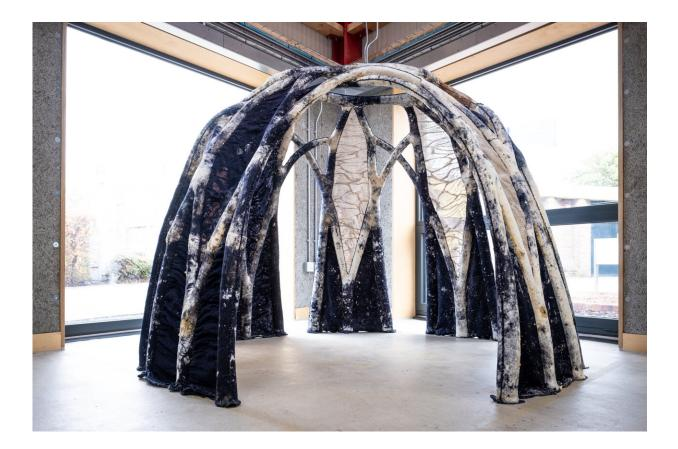
A 1.8m high, 2m diameter freestanding structure made of the BioKnit mycocrete using knitted formwork. Credit: Hub for Biotechnology in the Built Environment.
