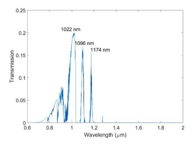
This figure from the study shows energy transmission by laser at different wavelengths from an altitude of 47 km. The 47 km altitude was chosen because, below it, there's less scattering of the beamed energy. There are likely enough windows in the atmosphere to allow lasers to transmit enough energy to operate a surface lander. Credit: Grandidier et al. 2023
