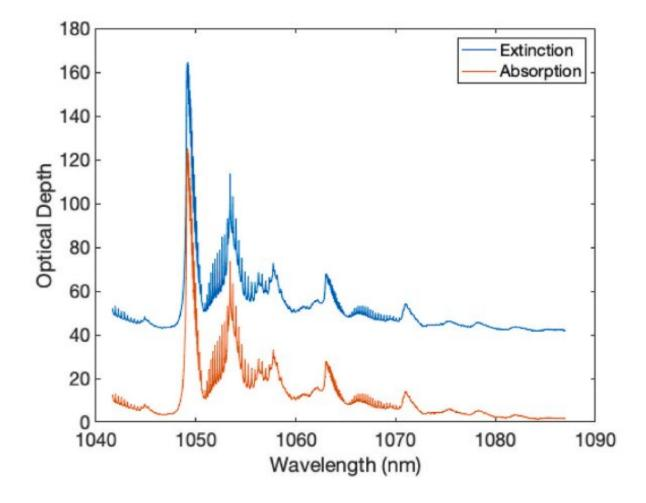
This figure from the study shows how Venus' atmosphere makes it difficult to beam power from above the clouds to the surface in microwaves. "In this spectral range, water vapour and CO2 are the only significant absorbing gases, while H2SO4 clouds/aerosols are the primary contributors to the extinction optical depths," the paper explains. Credit: Grandidier et al. 2023
