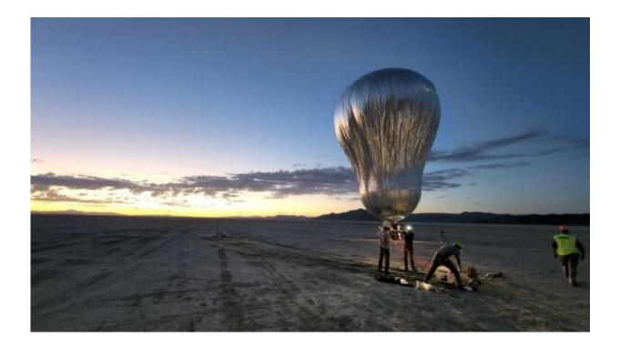
A prototype aerial robotic balloon, or aerobot, is readied for a sunrise test flight at Black Rock Desert, Nevada, in July 2022, by team members from JPL and Near Space Corporation. The aerobot successfully completed two flights, demonstrating controlled altitude flight. Credit: NASA/JPL-Caltech
