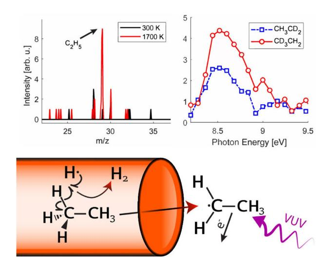
Graphical Abstract. We directly detect the ethyl radical intermediate in ethane pyrolysis for the first time, and reveal new insights into the reaction mechanism based upon our observations. This advance was enabled by a combination of isotopic microreactor studies, master equation based kinetics calculations, and
