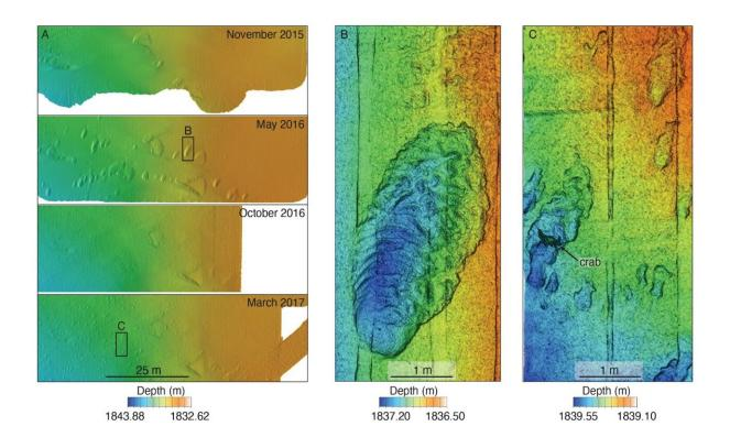
Four repeat surveys with MBARI's LASS sensor suite between November 2015 and April 2017 provided an incredibly detailed view of the changes to the floor of Monterey Canyon. The LASS combines various sensors, including sonar bathymetry at a resolution of five centimeters (two inches) (A) and lidar bathymetry (B and C) at a scale of one centimeter. Lidar data provide richer detail about the seafloor, revealing objects that are too small to be seen by sonar. Credit: Monica Wolfson-Schwehr, MBARI
