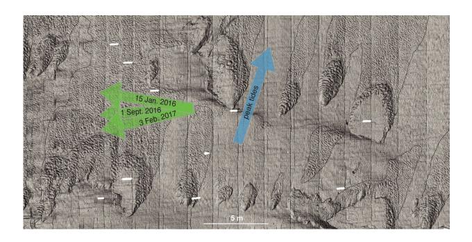
Lidar technology on MBARI's Low-Altitude Survey System (LASS) uses pulses of lasers to record the bathymetry, or underwater topography, on the seafloor at centimeter-scale resolution. Surveys with this sensor suite at a scour field 1,840 meters (6,037 feet) deep on the floor of Monterey Canyon revealed how turbidity currents (green) and tides (blue) affected the structure of the seafloor. Credit: Monica Wolfson-Schwehr, MBARI
