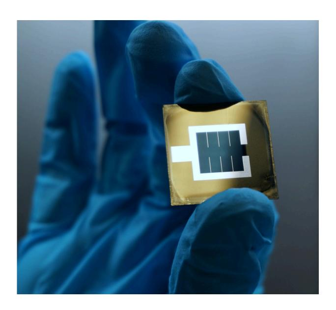
Photo of the perovskite/silicon tandem solar cell. The active area in the middle of the wafer is enclosed by the silver electrode. Credit: Johannes Beckedahl/Lea
