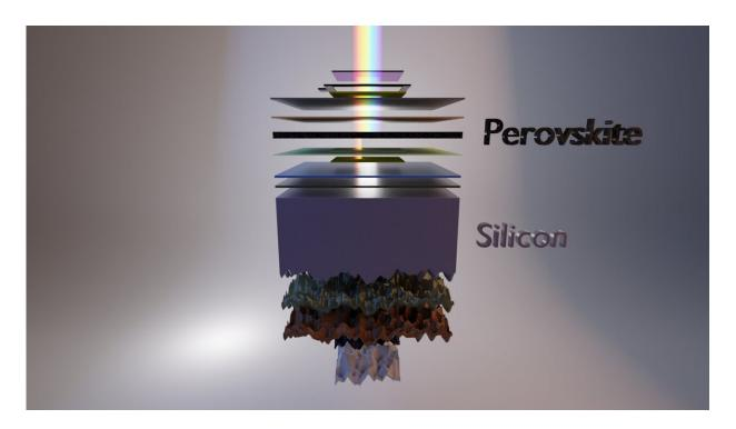
The illustration shows the schematic structure of the tandem solar cell with a bottom cell made of silicon and a top cell made of perovskite. While the top cell makes use of the "blue" components of the spectrum, the bottom cell converts the red and near-infrared light. Different thin layers optimize light use and minimize losses. Credit: Eike Köhnen/HZB
