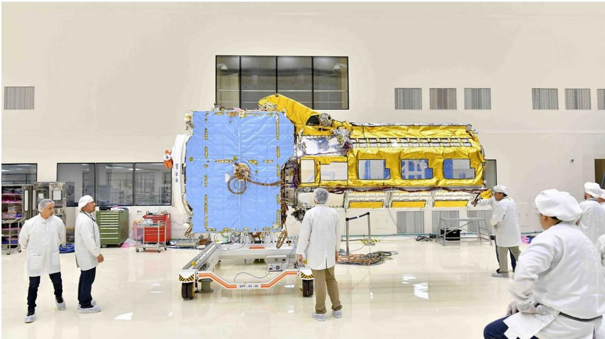
Engineers joined the two main components of NISAR—the spacecraft bus and the radar instrument payload—in an ISRO clean room in Bengaluru, India, in June. The payload arrived from NASA's Jet Propulsion Laboratory in Southern California in March, while the bus was built at the ISRO facility. Credit: VDOS-URSC
