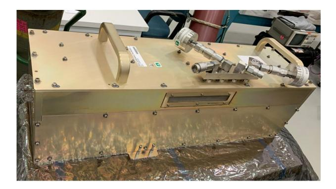
CM-HT in launch configuration showing silver colored launch accumulators and electro-magnetic interference screen. Credit: Science@NASA
