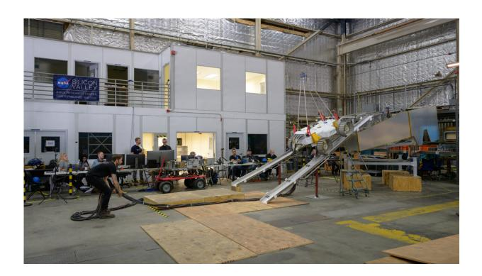
Antoine Tardy, VIPER rover egress driver, adjusts the cables that power and send commands to the VIPER test unit as engineers practice its exit/descent from the model Griffin lunar lander at NASA's Ames Research Center in California's Silicon Valley. Credit: NASA/Dominic Hart
