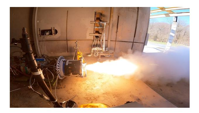
A development motor based on the second-stage solid rocket motor design for NASA's Mars Ascent Vehicle (MAV) undergoes testing March 29, at Northrop Grumman's facility in Elkton, Maryland. An important part of the NASA-ESA Mars Sample Return campaign, the MAV would be the first rocket fired off another planet. Credit: NASA
