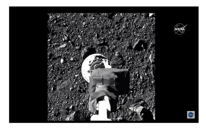
The robotic arm of NASA's OSIRIS-REx spacecraft makes contact with the surface of asteroid Bennu, as seen on an October 2020 video broadcast.
