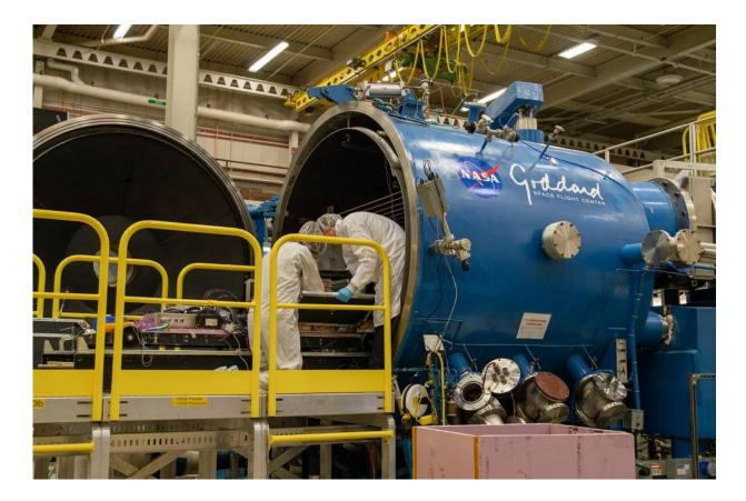
ComPair team members prepare the instrument for thermal vacuum testing. Once closed, the chamber will begin to simulate conditions the mission will experience during its balloon flight, which will take it to about 133,000 feet (40,000 meters), or nearly four times the cruising altitude of a commercial airliner. Credit: NASA's Goddard Space Flight Center/Scott Wiessinger
