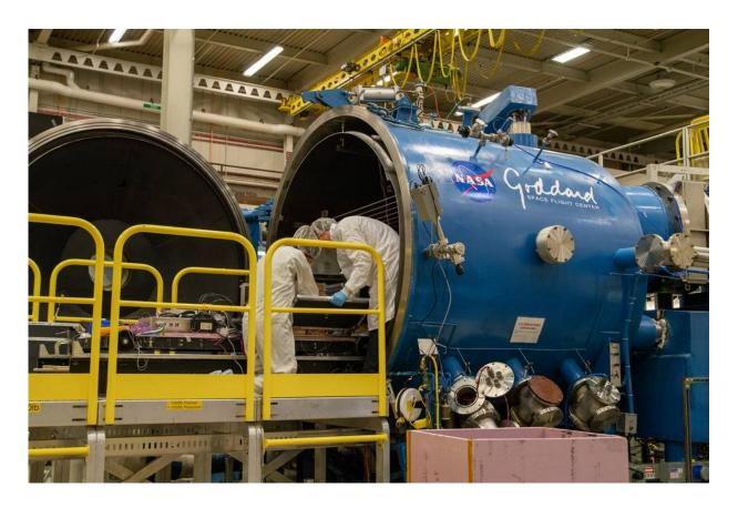
ComPair team members prepare the instrument for thermal vacuum testing. Once closed, the chamber will begin to simulate conditions the mission will experience during its balloon flight, which will take it to about 133,000 feet (40,000 meters), or nearly four times the cruising altitude of a commercial airliner. Credit: NASA's Goddard Space Flight Center/Scott Wiessinger
