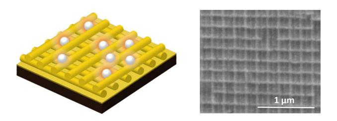
Sketch of SERS substrate with polystyrene beads (left) and scanning electron microscope image of SERS substrate used for the detection of nanoplastic (right). Credit: *Scientific Reports* (2023). DOI: 10.1038/s41598-023-37290-y
