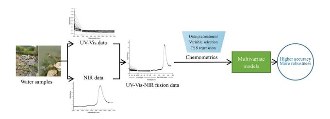
By fusing the data of surface water ultraviolet-visible spectra (UV-Vis) and near infrared (NIR) spectra, scientists realized fast and accurate detection of surface water quality. Credit: Xu Zhuopin
