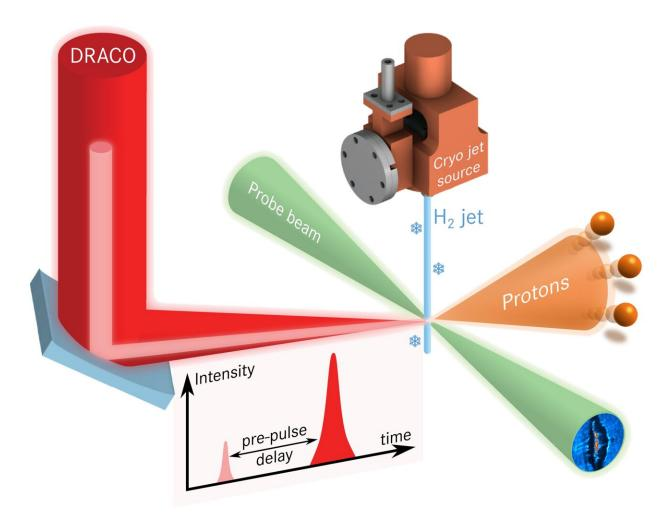
Schema of the experimental setup: By shooting an intense pulse (red) from the HZDR high power laser DRACO onto a continuously replenishing frozen hydrogen jet (blue), the researchers were able to massively accelerate protons over an extremely short distance (orange). They recorded the process with a synchronized optical laser pulse (green). Credit: SLAC National Accelerator Laboratory / G. Stewart
