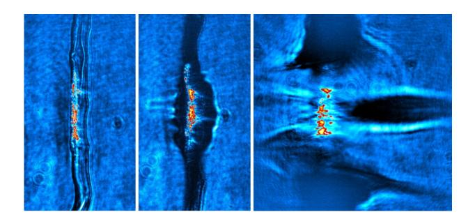
Shadowgraphs (blue) at the time of impact of the high-intensity laser pulse on the jet of hydrogen. A weaker light pulse sent in advance deliberately changed the hydrogen jet into three different initial states. Credit: HZDR
