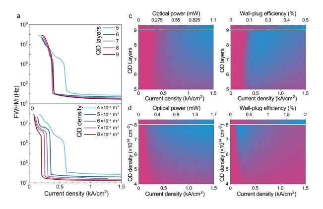
a,b Linewidth FWHM of the III-V/SiN QD laser as a function of the injection current density for different QD layers (a) and QD densities (b). c,d Colormaps of the output power (left) and wall-plug efficiency (right) as functions of the QD layers (c) and QD density (d). Credit: Emad Alkhazraji, Weng W. Chow, Frédéric Grillot, John E. Bowers, and Yating Wan
