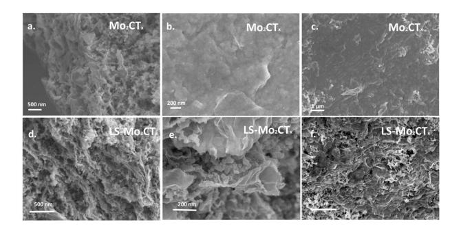
SEM images for  $Mo_2CT_x$  and LS- $Mo_2CT_x$  electrodes. (a) cross-section and (b,c) the morphology of  $Mo_2CT_x$ . (d) cross-section and (e,f) the morphology of LS- $Mo_2CT_x$ . Credit: *Small* (2023). DOI: 10.1002/smll.202208253
