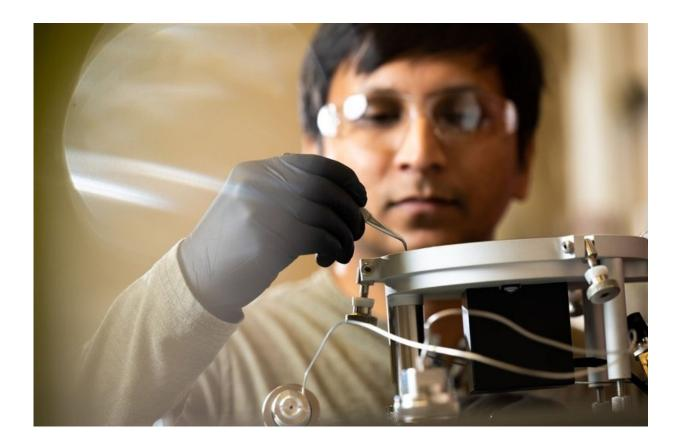
Scientists use the isotope ratio mass spectrometer at the EMSL user facility to analyze the ratios of different isotopes in organic and inorganic samples. Credit: Environmental Molecular Sciences Laboratory
