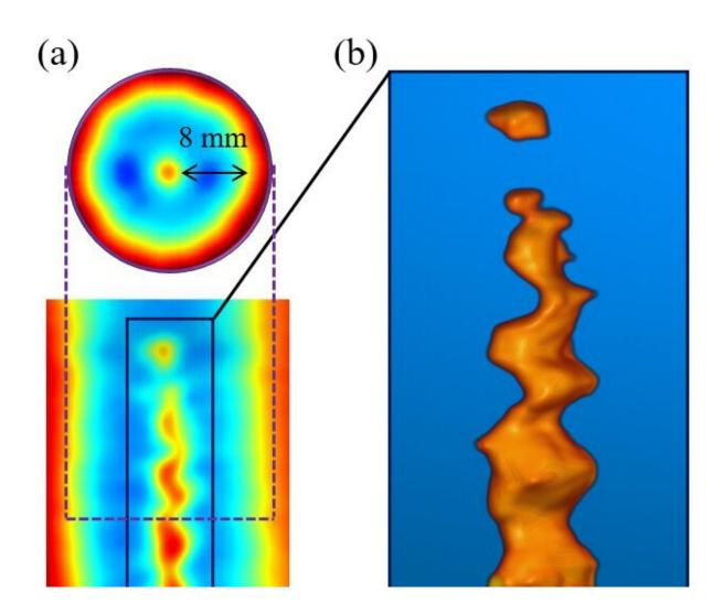
A new high-speed 3D imaging method can capture the complex behavior of the turbulent flames produced during combustion. Shown are two cross sections of the 3D density measurement at Z = 16 mm and X=0 mm, respectively(a) and the 3D iso-surface of the largest density gradient between the mixture and
