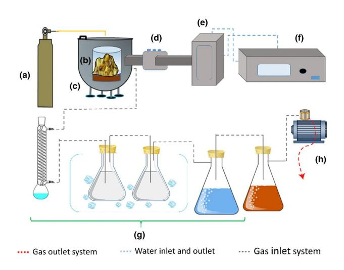
Microwave pyrolysis system used in the  $ZnCl_2$ -activated biochar synthesis. The system components are (**a**) nitrogen gas cylinder; (**b**) quartz beaker containing biomass of pineapple peel; (**c**) custom-made pyrolysis chamber; (**d**) tuner; (**e**) microwave generator; (**f**) microwave power controller; (**g**) condensers; (**h**)
