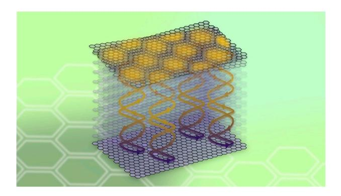
A University of Washington-led team has discovered that, by stacking a sheet of graphene onto bulk graphite at a small twist angle (top), "exotic" properties present at the graphene-graphite interface (yellow) can bleed down into the graphite itself. Credit: Ellis Thompson
