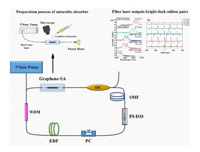
Structure of graphene mode-locked fiber laser and output of bright-dark soliton pairs. Credit: *Frontiers of Optoelectronics* (2023). DOI: 10.1007/s12200-023-00067-2
