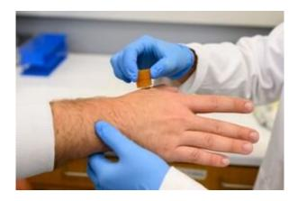
A WVU forensics researcher collects gunshot residue from a hand, using a sampling procedure in which carbon adhesive is mounted on an aluminum pin and plastic holder. Invisible gunshot residue can stick on the adhesive for further analysis. Credit: WVU Photo/Matt Sunday
