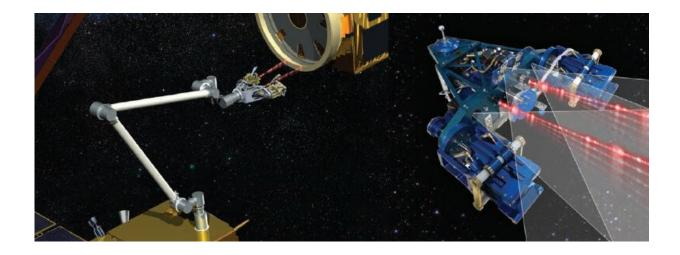
Artist impression of a servicing satellite using a capture tool and a vision system to approach and capture the launch adapter ring of a satellite. Credit: Astroscale
