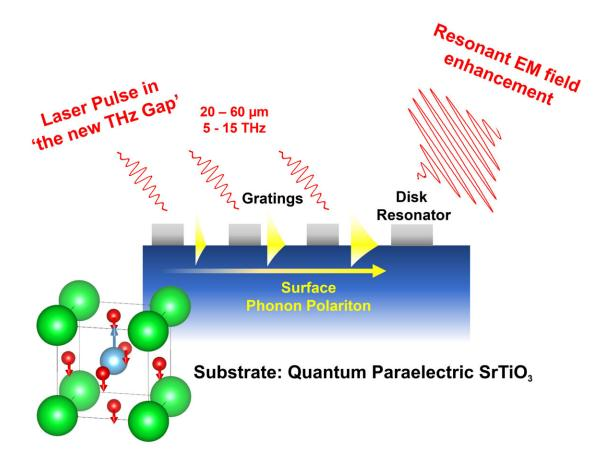
Illustration of a quantum paraelectric lens (cross-section) that focuses light pulses with frequencies from 5-15 terahertz. Incoming terahertz light pulses (red, top left) are converted into surface phonon-polaritons (yellow triangles) by ringshaped polymer gratings and disk resonators (grey) atop a substrate of strontium
