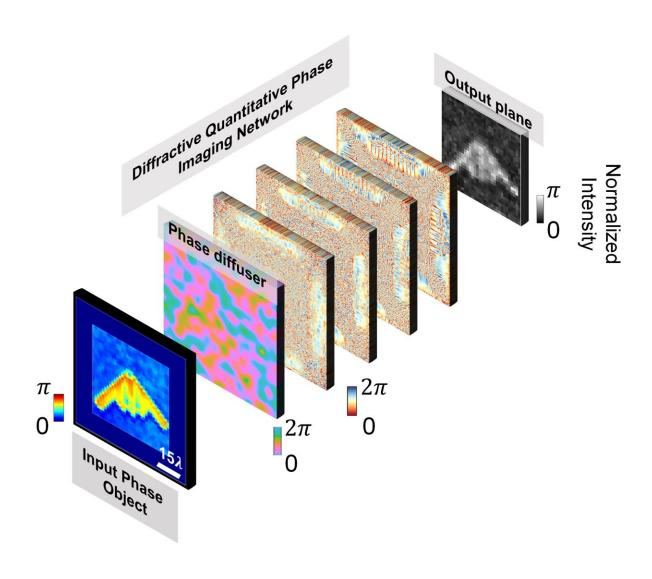
All-optical phase recovery and quantitative phase imaging (QPI) through random unknown diffusers using a diffractive optical network. The schematic of the
