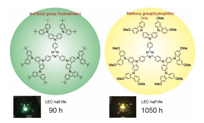
Second-generation dendrimers with tert-butyl (left) and methoxy groups (right) applied to light-emitting electrochemical cells (LEC). The lifetime of LEC devices using dendrimers with hydrophilic methoxy groups (right) is more than 10 times longer than that of hydrophobic dendrimers. Credit: Kyushu University/Albrecht Lab
