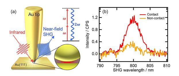
Figure 1. (a) Schematic representation of the experiment. Local SHG signal is enhanced by irradiating an infrared laser pulse into the plasmonic nanogap between the gold tip and the gold substrate. (b) SHG spectra obtained with (red) and without (orange) plasmonic nanogap, indicating that the SHG signal is enhanced only when the tip is brought closer due to the plasmonic enhancement effect unique to the tip-substrate nanocavity. Credit: Toshiki Sugimoto
